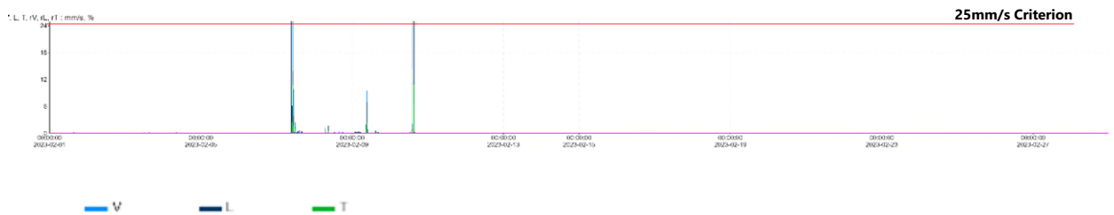
Figure 7-4 - Real-time vibration monitoring results at the Hickson Road wall, February 2023 (Monitor 1)
