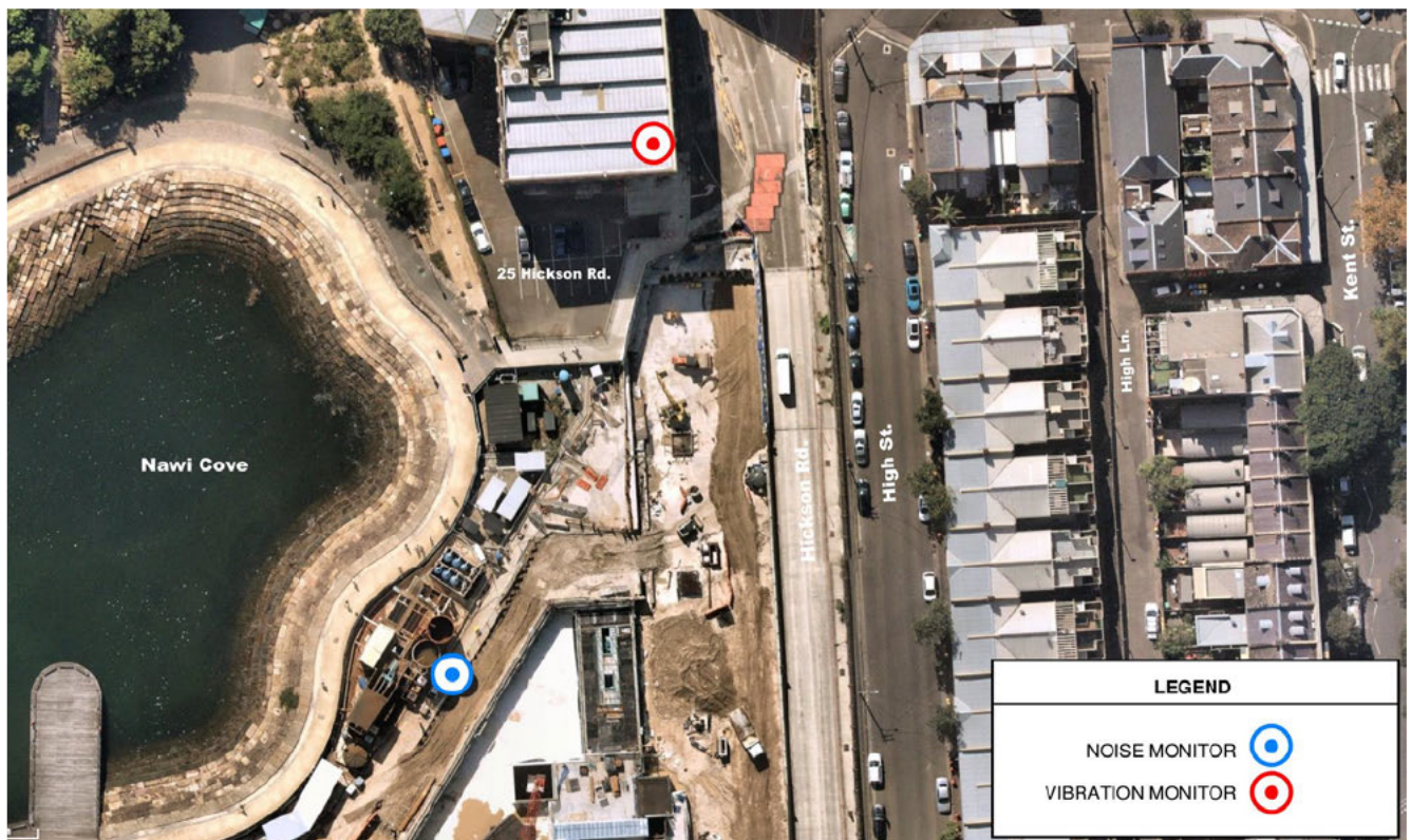
Figure 2 – Location of on-site Noise and Vibration monitors
